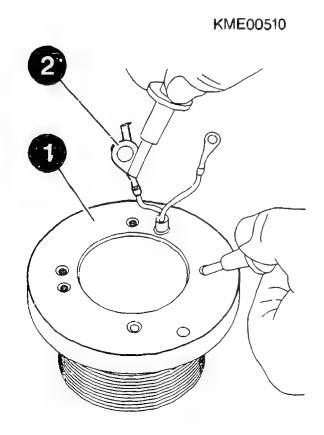
CHECKING AND REPAIRING ALTERNATOR Checking pole body (resistance) Use alternator tester to measure pole body resistance between connections (1) and (2). Pay attention to measuring range on measuring instrument. Resistance value: 1,9...2,1 Ohm
